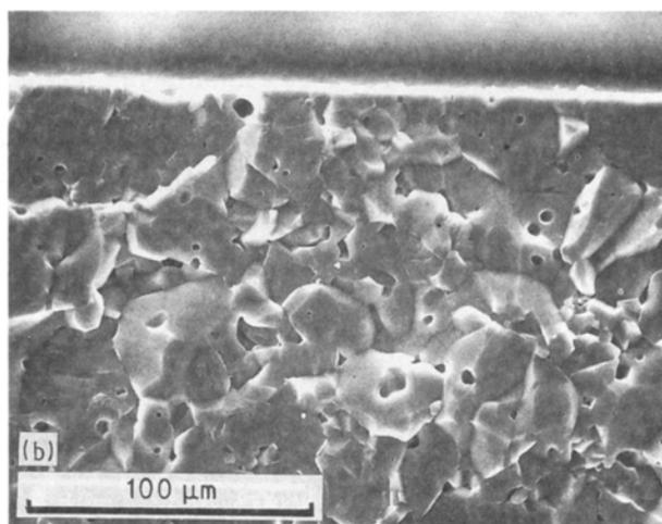
Figure 5 Fracture surfaces of uncoated polycrystalline alumina, (a) 95% and (b) 99.5%. Both alumina failed intergranularly.
