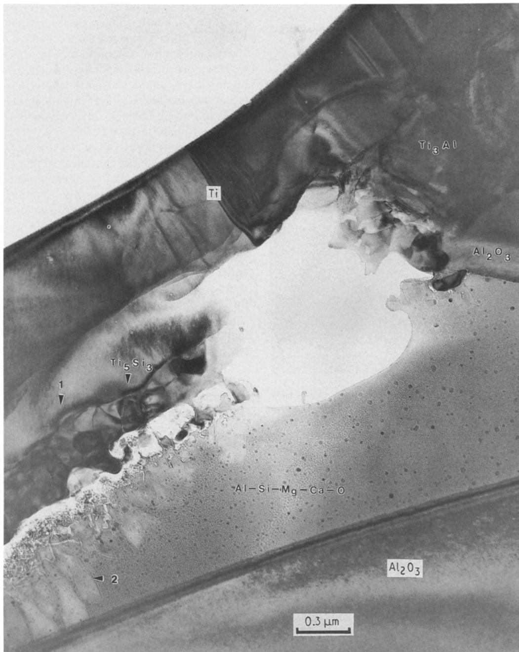
Figure 8 Interface microstructure of titanium/95% polycrystalline alumina. Reactions at the interfaces of titanium/alumina and titanium/-grain-boundary glassy phase resulted in an  $Ti_3Al$ -type phase and  $Ti_5Si_3$ , respectively. Arrow 1 shows the strain contour in the vicinity of  $Ti_5Si_3$ . Another second phase, depleted of calcium from the glass composition, formed at the interface, arrow 2.
