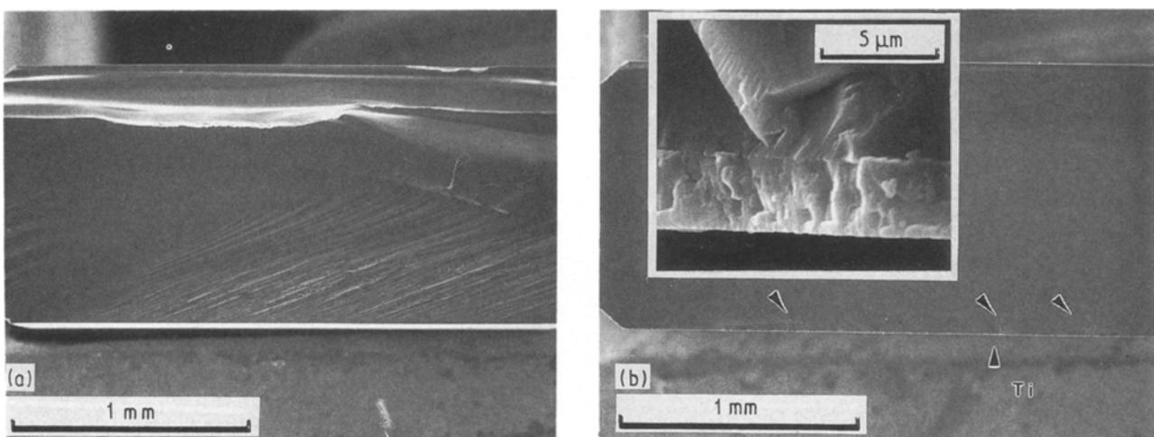
Figure 7 Typical fracture surfaces of sapphire, (a) uncoated and (b) titanium-coated. Cracking was initiated at a chamfered corner of uncoated sapphire, whereas more than one potential flaw for crack initiation was observed (see arrows) from the titanium-coated sapphire.
