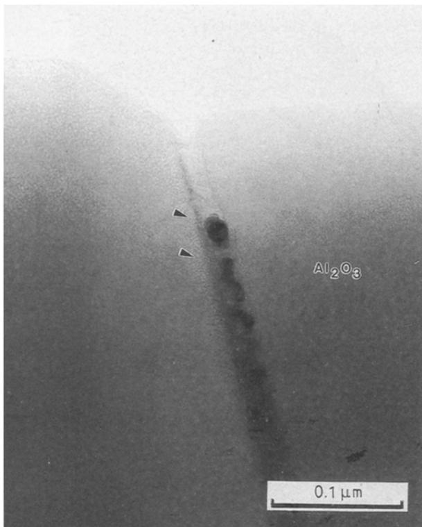
Figure 9 Interface microstructure of titanium/grain-boundary glass phase of 99.5% polycrystalline alumina. Reaction between titanium and 99.5% alumina resulted in spherical phases of 0.01–0.02  $\mu\text{m}$  diameter. The titanium-coating layer which was on the top of the grain boundary was removed during the ion-milling process.
