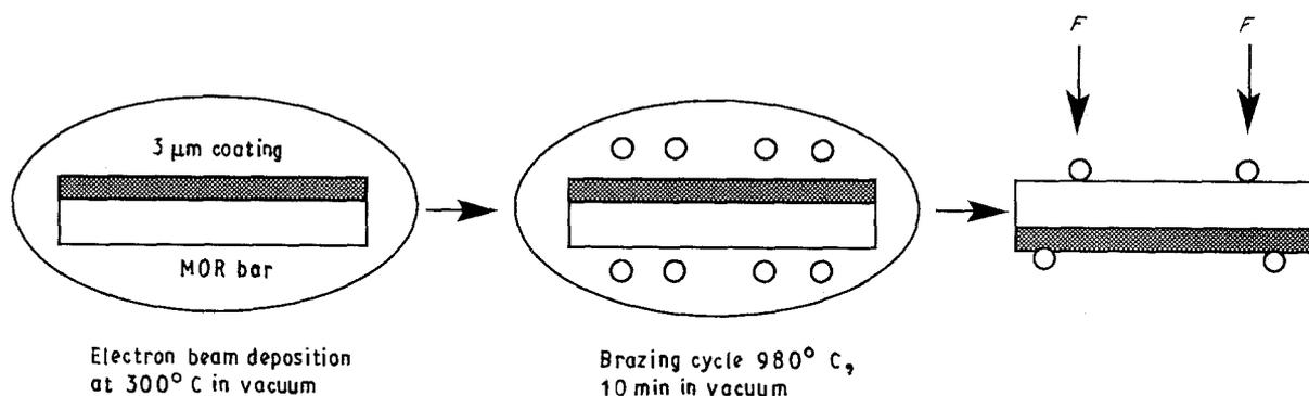
Figure 1 Procedure to evaluate the effect of coating on the MOR strength of ceramic materials. Coated samples were heated at 980  $^\circ\text{C}$  for 10 min prior to four-point bend test.
