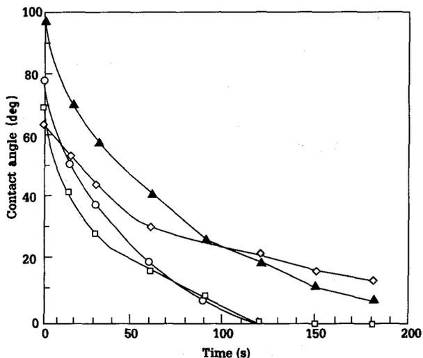
Figure 2 Wetting angles versus time at 1000°C with an Au-18% Ni alloy: alumina with reactive coatings showed the improved wetting behaviour of an Au-18% Ni alloy compared to the uncoated alumina (> 90°). Coating (▲) titanium, (□) zirconium, (○) tantalum, (◇) hafnium.
