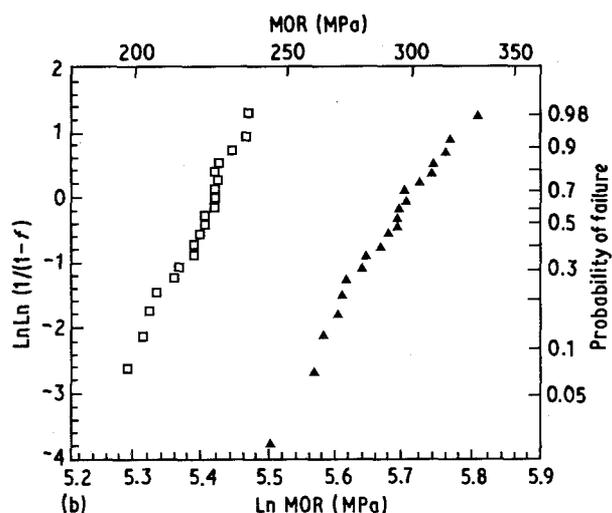
Figure 3 Weibull distribution of the MOR strength of (a) 99.5% and (b) 95% polycrystalline alumina. The presence of reactive coatings reduced the MOR strength of the alumina by 15%–25%. Coatings; (▲) uncoated, (□) titanium, (○) zirconium, (◇) hafnium, (+) tantalum.
