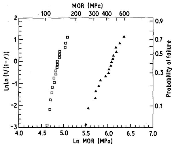
Figure 4 Weibull distribution of the MOR strength of sapphire. Titanium coating reduced the MOR strength of the sapphire by 65%. (▲) uncoated, (□) titanium coated.
