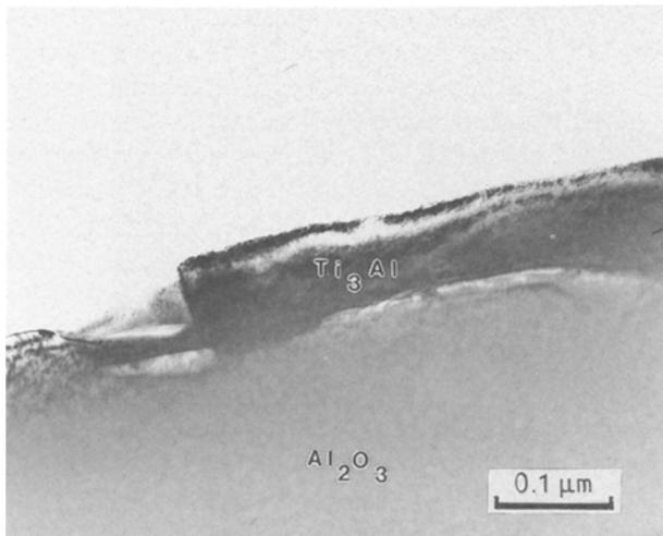
Figure 10 Interface microstructure of titanium/sapphire. Titanium reacted with sapphire and formed a  $\text{Ti}_3\text{Al}$ -type phase. The titanium-coating layer on the top of a  $\text{Ti}_3\text{Al}$ -type phase was removed during sample preparation.
