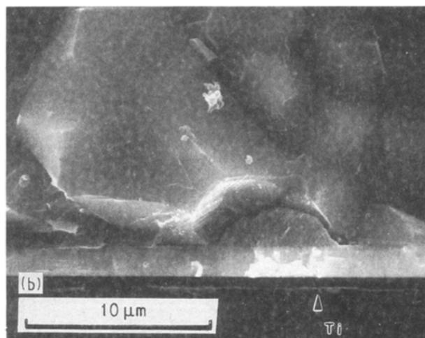
Figure 6 Fracture surfaces of titanium-coated polycrystalline alumina, (a) 99.5% and (b) 95%. The fracture surfaces of the coated and uncoated bars were similar. Note the strong adhesion between titanium coating and alumina.
